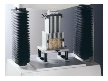
range to accommodate interchangeable load cells from 0.5kg up to 750kg (for twin column models), allowing attachment of the widest range of probes, fixtures and attachments in the field.
